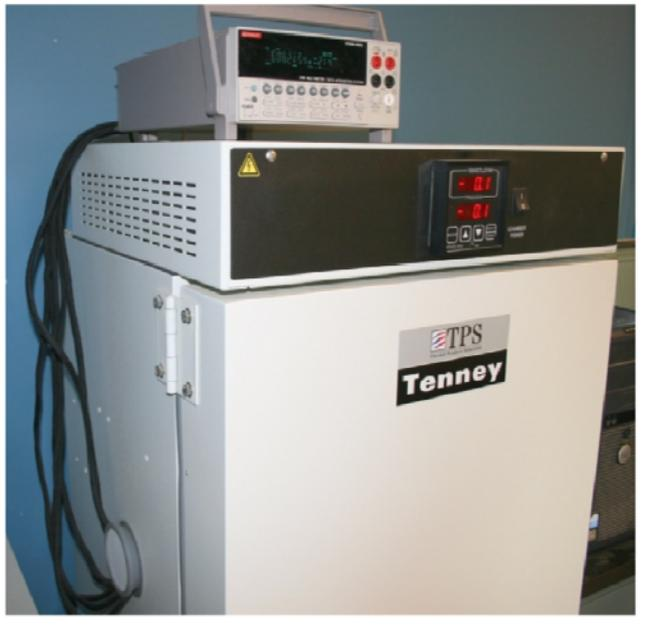
All peltier plates and thermistor are wired through serial port and connected to multimeter.
